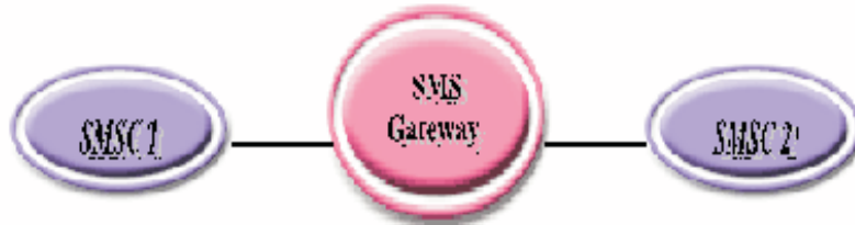
Figure 6 An SMS gateway acts as an interface between two SMS centers.
