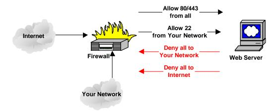
Firewalls filter the traffic exchanged between networks, enforcing each network's access control policy. Often, a firewall defends an inside "trusted" network from attack by "untrusted" outsiders. Firewalls ensure that only authorized traffic passes into and out of each connected network. To avoid compromise, the firewall itself must be hardened against attack. To enable security policy design and verification, a firewall must also provide strong monitoring and logging.
