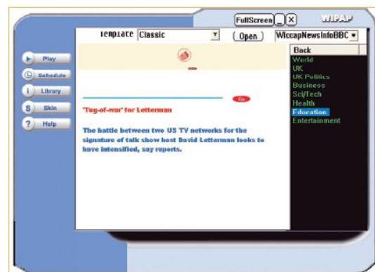
Figure 4. The Wicap system at runtime. The buttons on the left correspond to frequently used functions, the center panel shows the active view's content, and the list on the right shows the view's skeleton.
